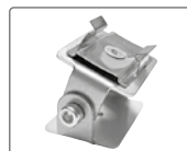
FL/CLIP-Adjustable** (35,5x19x22 mm) Federstahl / stainless spring steel verstellbarer Montagewinkel, 75° zu beiden Seiten neigbar adjustable mounting clip, 75° on both sides
